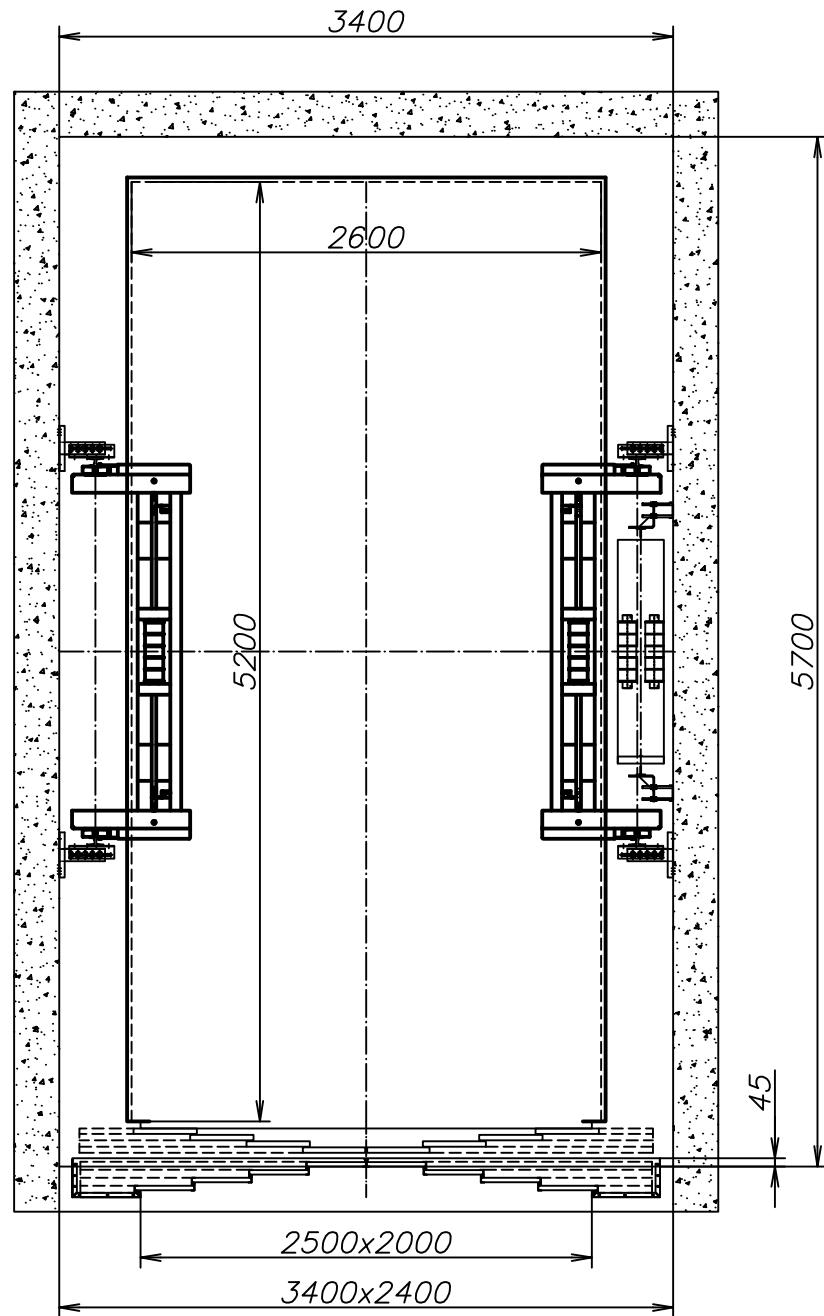
1. Deviations of the hoistway width and depth from the nominal sizes
